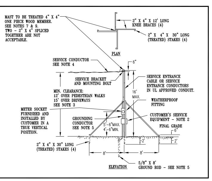
FIG. 11 - TEMPORARY SERVICE FROM OVERHEAD FACILITIES
