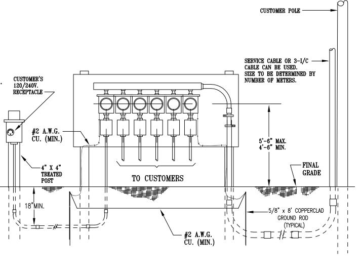
FIG. 2A MOBILE HOMES AND TRAILER COURTS SINGLE PHASE, 3 WIRE, 120/240 VOLT SERVICE - 100 AMP. OR 200 AMP.
