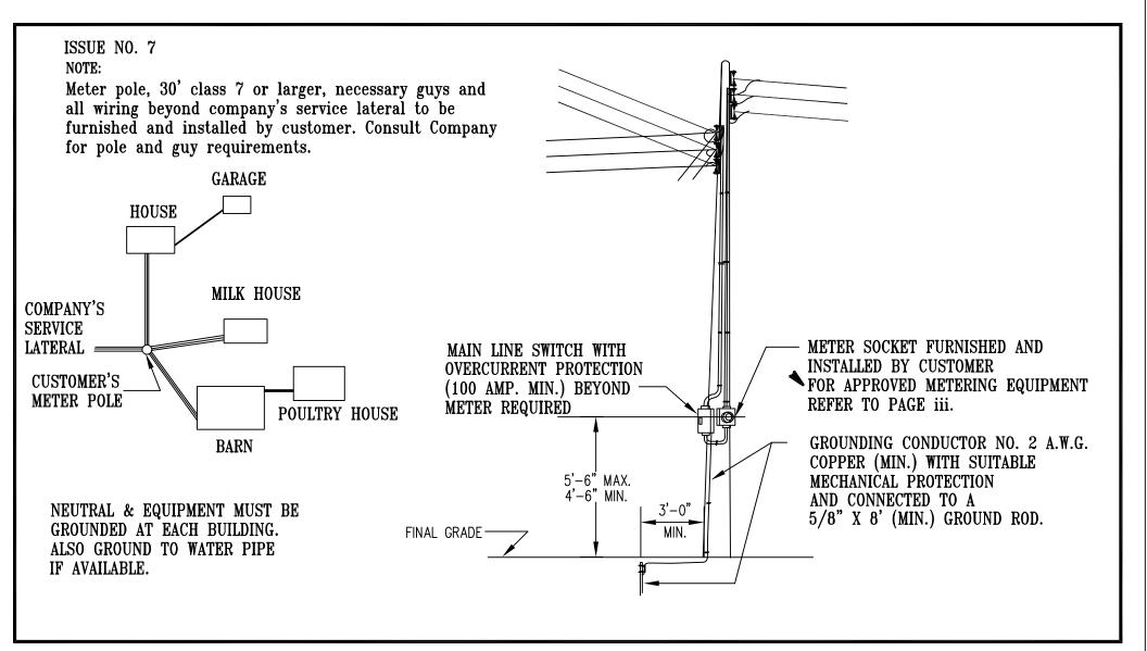
FIGURE 2 OUTDOOR INSTALLATION ON A POLE - ONE METER
