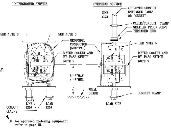
FIG. 4A METER SOCKET MTG. DEVICES / WIRING METHODS /OUTDOOR SELF-CONTAINED METERS 200 AMP. MAX. THREE PHASE, 4 WIRE, 120/208 VOLT, WYE CONNECTED.
