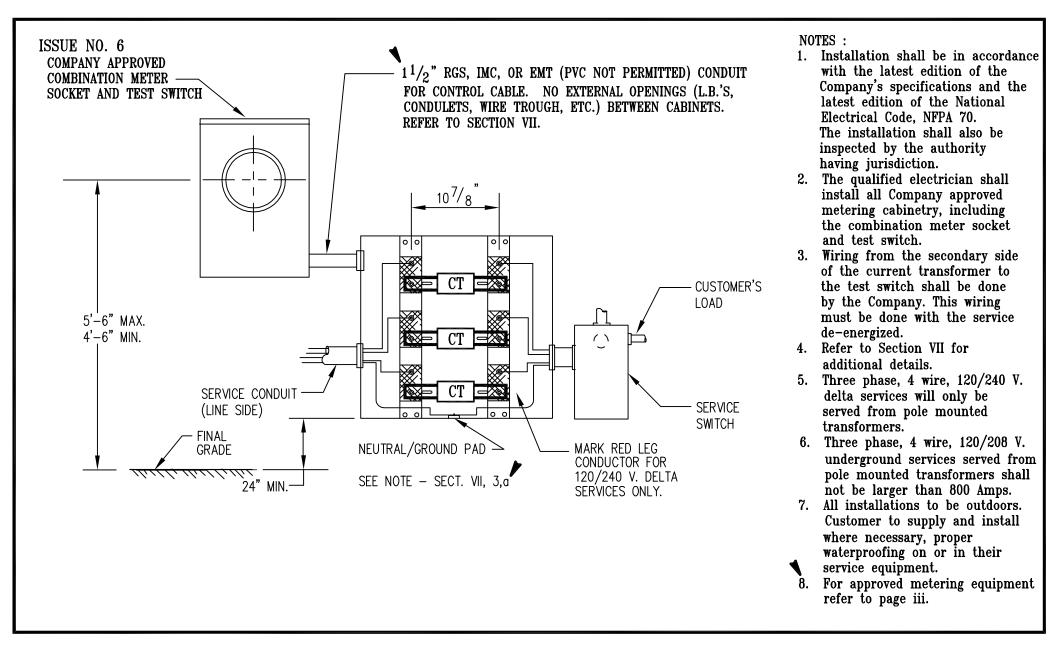
FIG. 6 INSTRUMENT TRANSFORMER RATED METER COMBINATION METER SOCKET AND TEST SWITCH THREE PHASE, 4 WIRE, 120/208 VOLT OVERHEAD SERVICE FROM 201 TO 400 AMPS. THREE PHASE, 4 WIRE, 120/208 VOLT UNDERGROUND SERVICE FROM 201 TO 1200 AMPS. (SEE NOTE 6) THREE PHASE, 4 WIRE, 120/240 VOLT OVERHEAD SERVICE FROM 300 TO 400 AMPS. (SEE NOTE 5) THREE PHASE, 4 WIRE, 120/240 VOLT UNDERGROUND SERVICE FROM 300 TO 600 AMPS. (SEE NOTE 5)
