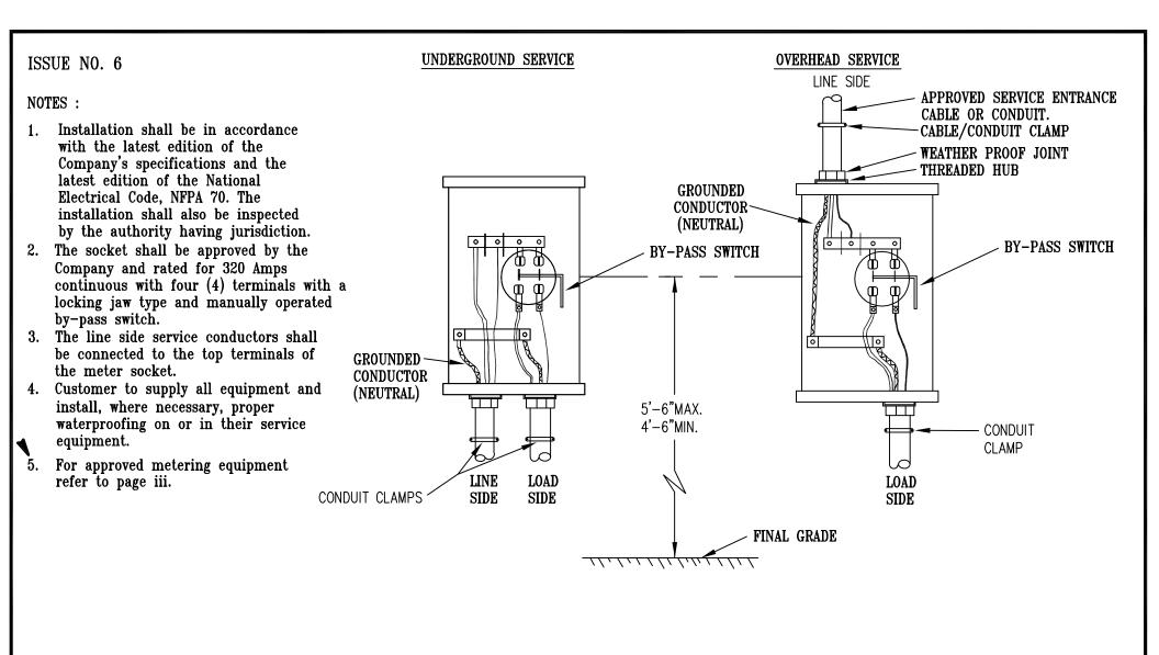
FIG. 4 – METER SOCKET MTG. DEVICES/WIRING METHODS/OUTDOOR SELF-CONTAINED METERS/300 AMPS. MAX.
