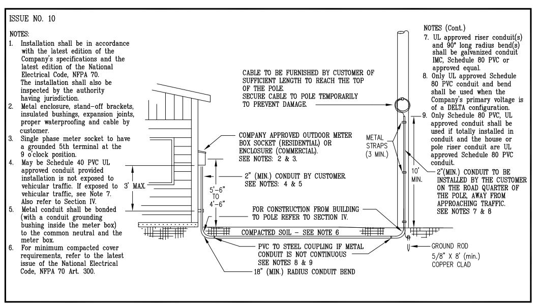
FIG. 8 – TYPICAL UNDERGROUND SERVICE CONNECTION BELOW 600 VOLTS FROM OVERHEAD LINES NOTE: CALL BEFORE YOU DIG. SEE PREFIX PAGE iv FOR THE UNDERGROUND MARK OUT NUMBER IN YOUR AREA.
