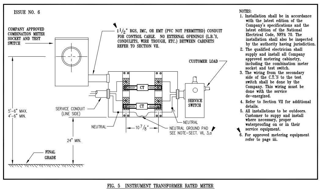
COMBINATION METER SOCKET AND TEST SWITCH
