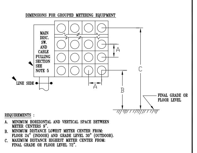
FIG. 3 - GANGED METER SOCKET CONFIGURATIONS/INDOOR SELF-CONTAINED METERS
